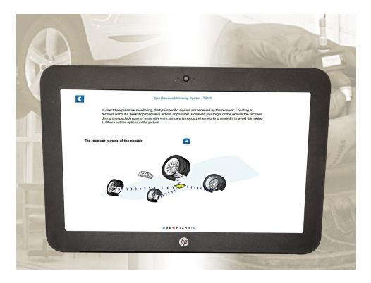
There are two main types of TPMS - Direct and Indirect Pressure Monitoring. In this training module you will learn the basics of both of these systems and how they operate, including:
